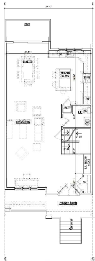
UNIT TYPE B (INTERIOR UNIT) FIRST FLOOR PLAN SCALE: 1/4" = 1'-0" LIVING AREA: 648 SF
