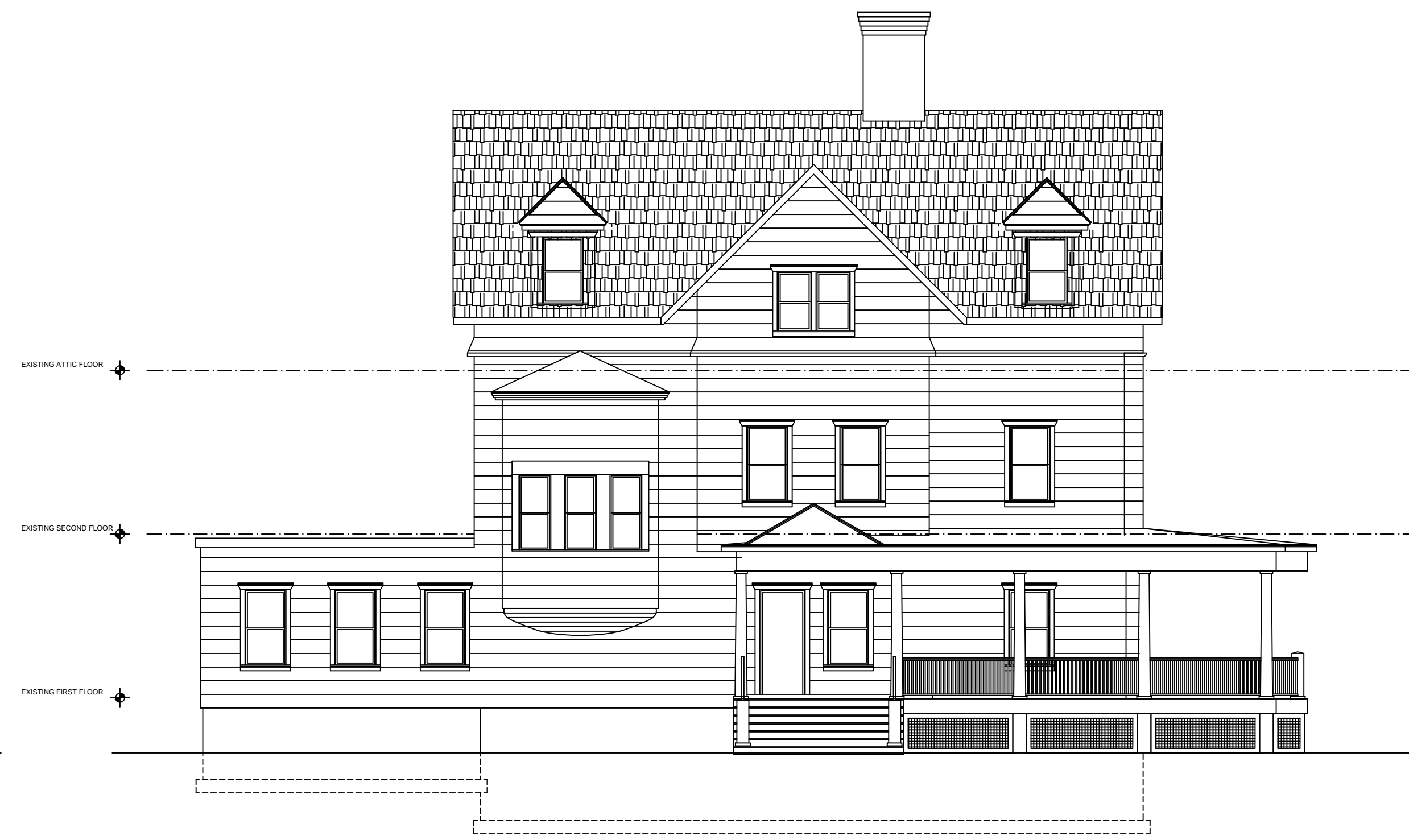
Existing Front (West) Elevation ① SCALE: 1/8" = 1'-0"
